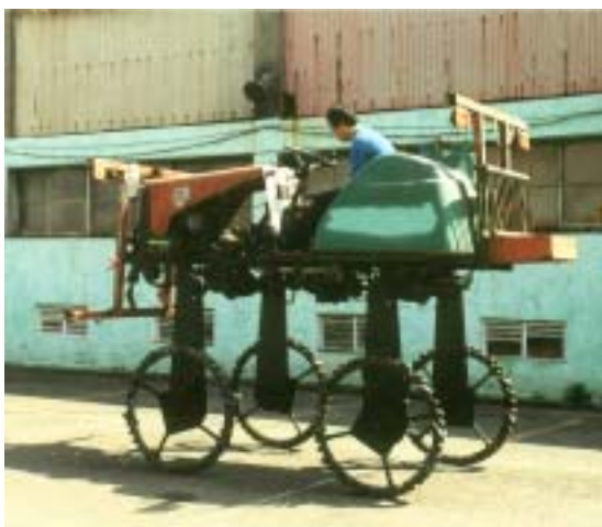
圖 8. 改裝後高架式工作母機之外貌 Fig 8. View of the high-clearance deleafing machine for Pachira Macrocarpa plants
