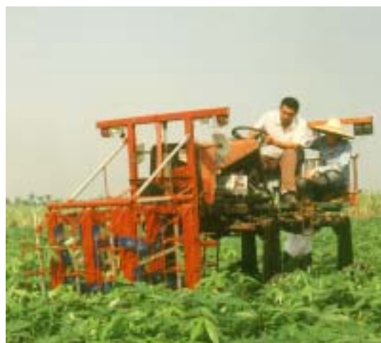
圖 9. 去葉機田間測試情形 Fig 9. Field testing of the deleafing machine for Pachira Macrocarpa plants
