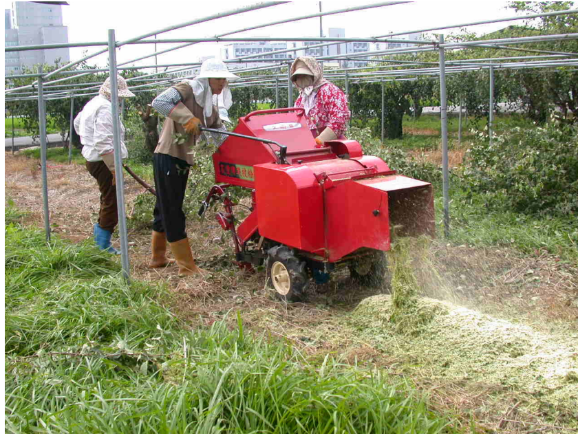
圖 5. 研製之自走式果樹殘枝粉碎機田間作業 Fig 5. Field operation of the developed self-propelled pulverizer for orchard residual branches
