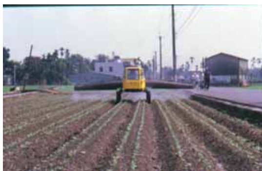
圖 2.紅豆採用氣輔桿式噴藥車防治病蟲害 Fig 2. Using automatic boom sprayers controlling disease and insect- pests
